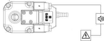
4. Connect the power supply to the drain alarm connector to close the circle. Replace the connector and tighten the connector screw (max. torque 0,3 Nm). *Make sure the gasket is secured properly to ensure IP65(NEMA4) rating.*
