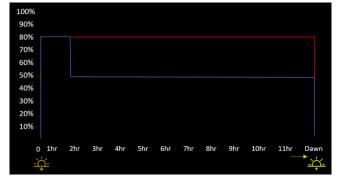
For the first 2 hours the product runs at 80% output, the next 12 hours after the first 2, it will run it at 50% idle & 80% when motion is sensed until dawn. The motion sensor output stays on for 30 seconds unless motion is still detected.
