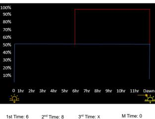
1<sup>st</sup> Power: 50% 2<sup>nd</sup> Power: 100% 3<sup>rd</sup> Power: 50% M Power: 0%
