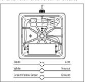
5. Replace the metal plate and the lens, make sure no wires are pinched when replacing parts.
