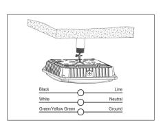
3. Screw the Conduit into the hole on top of Canopy light. Installation done.
