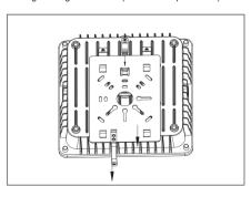
2. Connect the wires threaded from conduit and Canopy, Black wire for Line, White for Neutral, Yellow Green for Ground.
