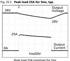
Output voltage dips from 24V to 20V.
