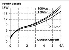
Fig. 9-4 Losses vs. input voltage, 24V, 5A
