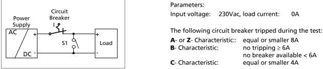
Test 2: Short circuit with S1 on the load end (additional impedance included; represents longer load wire length).
