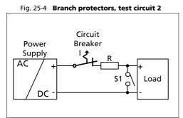
Parameters: Input voltage: 230Vac, load current: 0A
