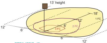
OPTICAL HEIGHT = 13' 6' BETWEEN AXIS TICK-MARKS TILT = 0° FROM NADIR
