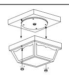
\*Push the shade straight into ceiling pan, and then twist the two mounting screws tightly.
