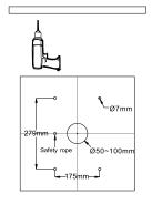
Fix another side of safety rope on the ceiling, then connect the wire of fixture to main power source according to local electrical connection code, make sure the wire joints are well protected, after that, fix the fixture on the ceiling with accessory screws.
