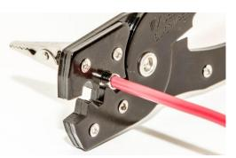
**3)** Important! Align the clip such that the "tooth" of the crimper faces the bottom of the clip. Squeeze tight on the crimpers handles.
