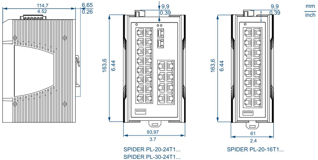
Figure 5: Dimensions of device variants SPIDER PL-20... and SPIDER PL-30...
