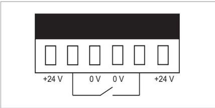
A diagram of a 6-pin connector. The top half is a solid black rectangle. Below it are six rectangular pins. The first and last pins are labeled '+24 V'. The second and third pins are labeled '0 V'. The fourth and fifth pins are also labeled '0 V'. A switch is shown below the second and third pins, with a line connecting it to the '0 V' label between the fourth and fifth pins. | 1   | + 24 V DC |
