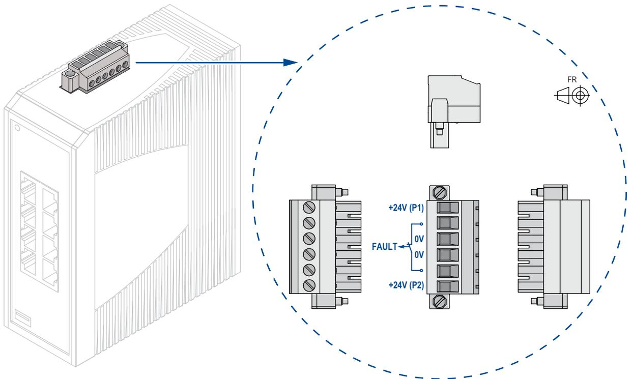
Figure 2: 6-pin terminal block, characteristic value HH
