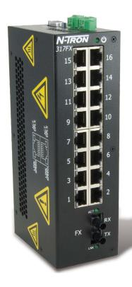
The 317FX-N simplifies plant wiring by eliminating the need to bring data acquisition and control connections back to a climate controlled environment. The switch has extended operating specifications to meet the harsh needs of the industrial environment, including extended temperature rating, extended shock and vibration specs, redundant power inputs, and a high MTBF (greater than 2M hours).
