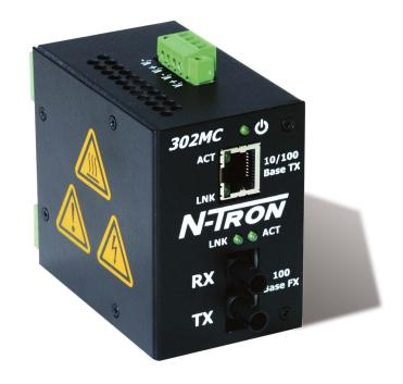
The 302MC has extended operating environmental specifications to meet the harsh needs of the industrial environment. For cost savings and convenience the media converter can be DIN-RAIL mounted alongside Ethernet I/O or other Industrial Equipment. The unique compact size provides a small footprint, conserving space in the most critical dimension. The 302MC can also be panel mounted
