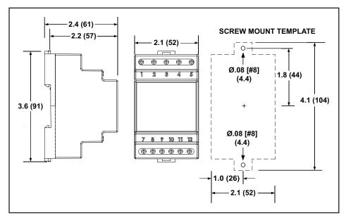
Fig. 1 Dimension Drawing: Inches (mm)
