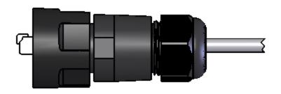
STEP 3.) Push grommet back into the "fingers" of the shell. Rotate cable 90 degrees and pull it back into connector until it stops. With slight tension on cable, tighten dome nut (3.75Nm recommended).
