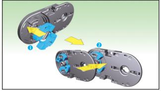
Insert BR unit to each side band, connect the side bands as many as you need, then do the same process to the other side of side band.
