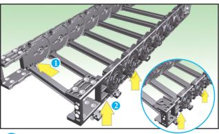
Attach frames to one side groove on the side band. and then the other side.
