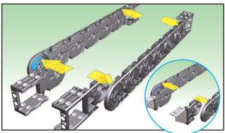
Assemble the end brackets on both ends using the same method.
