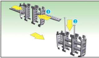
For ST072N, 095N, 120N, and 150N, connect the pin of separator in hole of divider after inserting separator in hole of divider, For ST044N and ST055N, separator fixing pins are not used.
