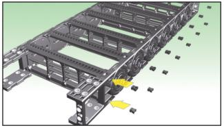
Insert frame pins to secure the frames and complete carrier. (ST072N, 095N, 120N, 150N are applied with frame pin, and ST044N, 055N are Hinge Type or Hook Type without frame pin.)
