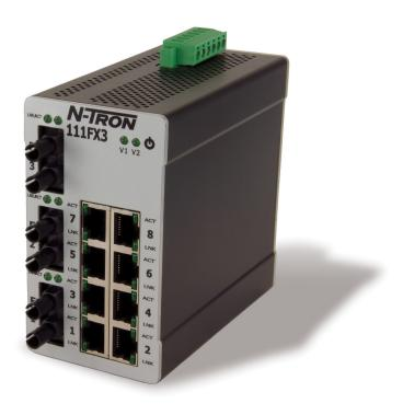
For fiber optic networks, the 111FX3 supplies three 100BaseFX ports. These connections provide vital support for applications where EMI immunity or communication over long distances (up to 80 km) is required. N-Tron offers singlemode or multimode installations, as well as SC- or ST-style connectivity.
